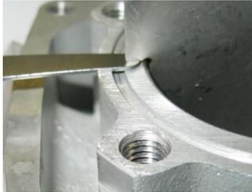
14. Exhaust valve. If the piston is moved in direction top of cylinder and first time covering completely the exhaust port, it must be possible to insert the exhaust valve gauge (ROTAX part no. 277 030) until it stops at the surface of the cylinder (a feeler gauge of 0.05 mm must not be possible to fit in).
