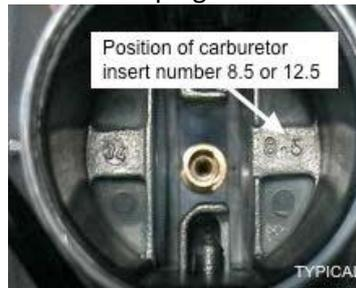
25. Angular bore: Plug gauge 0.60 may not fit. (8.5 Carburettor Insert only) (Use jet gauge set ROTAX part no. 281 920)
